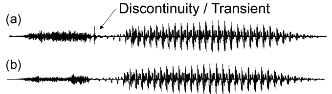
Fig. 8. (a) Speech signal for the utterance [fva] using a single lumped kinetic resistance. (b) Same utterance synthesized with the proposed loss model.
