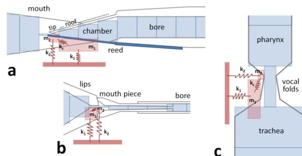
**Figure 2** – Two mass approximation of the mechanical part of the sound source (red and light red structures: springs and masses) and tube section model of the filter (light blue boxes represent sections of cavities) for clarinet (a), trumpet (b) and voice (c). The smallest tube section represents the reed tip narrowing for clarinet, the lip narrowing for trumpet and the glottis narrowing for voice.
