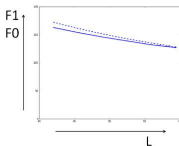
**Figure 6** – Variation of pitch ( $F_0$ ) as function of bore or tube length  $L$  for a clarinet. Beside pitch  $F_0$ , resulting from the self-oscillating source model (solid blue line), the calculated lowest resonance frequency of the bore  $F_1$  is displayed (dashed blue line).
