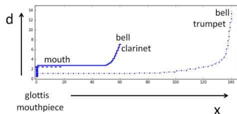
**Figure 1** – Geometrical models used for our numerical simulations for vocal tract (a “technical” schwa-vowel is articulated, dashed line), for a Bb-clarinet (all tone and register holes are closed, solid line) and for a Bb-trumpet (no valve is pressed, dash-dotted line); x-axis: length x of instrument in cm; y-axis: diameter d of bore or tube in cm.
