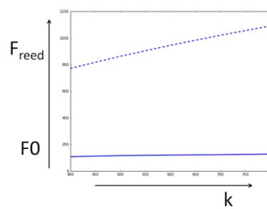
**Figure 7** – Variation of pitch ( $F_0$ ) for clarinet as function reed stiffness if of bore or tube length is constant. Beside pitch the eigenfrequency of the source system  $F_{reed}$  is displayed as well (dashed line).
