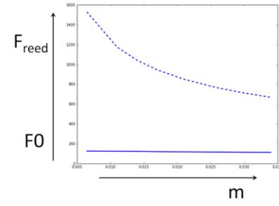
**Figure 8** – Variation of pitch ( $F_0$ ) for clarinet as function reed mass if of bore or tube length is constant. Beside pitch the eigenfrequency of the source oscillator  $F_{reed}$  is displayed as well (dashed line).
