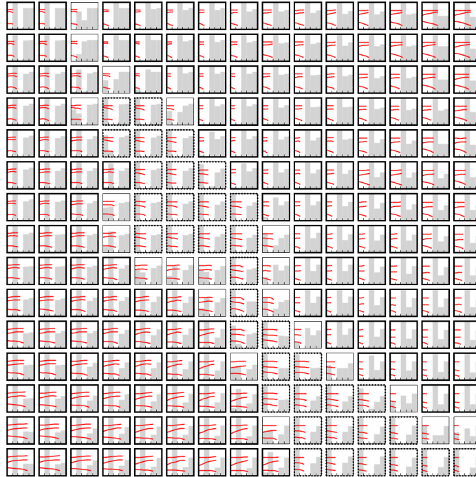
Fig. 5. Diagram of motor plan and auditory link weight values after proto-consonantal babbling training for each neuron within the vocalic phonetic map (15x15 neurons). Link weight values are given for five motor plan parameters within each neuron box. First three columns: vocal tract organ which performs the closing gesture (labial, apical, dorsal); two last columns: back-front value (fourth column) and low-high value (fifth column) of the starting vowel within the VC-sequence. Link weight values are given for three auditory parameters: bark scaled F1, F2, and F3 (formant transitions within each neuron box). Outlined boxes: see text.
